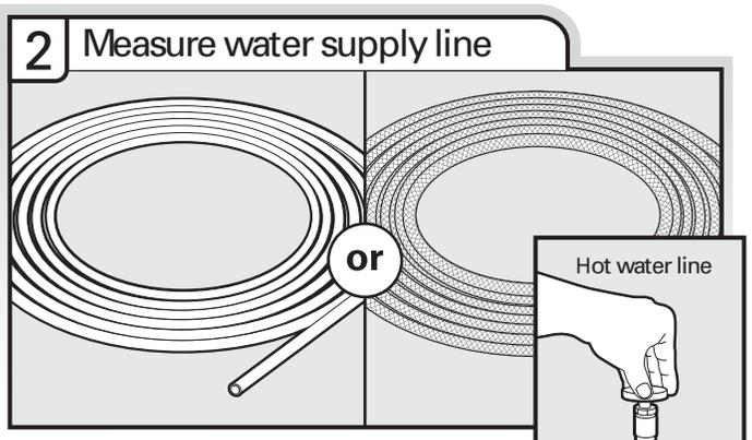
Measure overall length of copper tubing or flexible braided water supply line. Attach to the hot water line using a connection configuration that is in compliance with local codes and ordinances. The water line to the dishwasher should have a manual shutoff valve.
